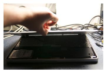
Once all screws have been removed, you should notice the panel begin to move ever so slightly upward, so you can now reach into the small crevice to lift the panel with ease. Unlike previous models, you will not have to worry about any data ribbons or small cables being attached to the bottom panel. You can simply lift it up with no concern.
