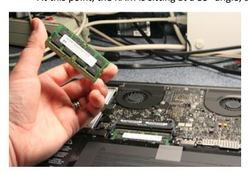
Do the exact same thing for the next stick underneath, and when you're ready, simply reconnect your new sticks by doing the same thing in reverse, ensuring the teeth are properly aligned with the grooves and pressed in, and finally press them down so they snap back into place.
