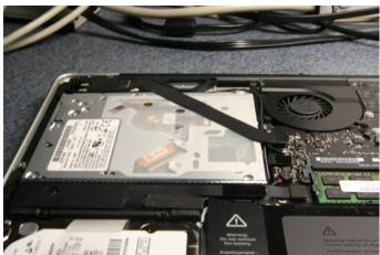
As you observe closely, you'll see the ribbon cables that are attached to both the optical drive and the hard drive. These cables are known as the **A1278** data cables. These cables are an example of a fragile component that you'll want to be very gentle with as you disconnect them.
